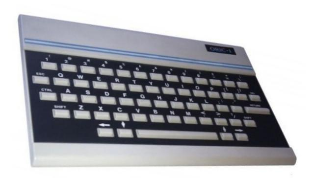
Like many home computers of the early 80's, the Tangerine Computers Oric-1 does not have a power switch. When you need to reset the computer you have to remove the power plug from the computer. This wears out the power socket on the computer causing intermittant power and eventually failure.
