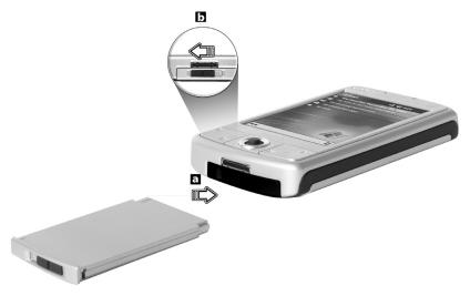
**NOTE:** To take the battery pack out, first slide the battery release switch to the unlocked position, then pull the battery pack out of the bay.
