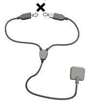
**NOTE:** If you are using the 3-in-one sync cable (an optional accessory), please do not plug the USB host into the USB client.
