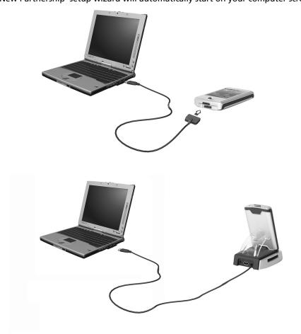
Plug the USB client connector into a USB port on your computer.
